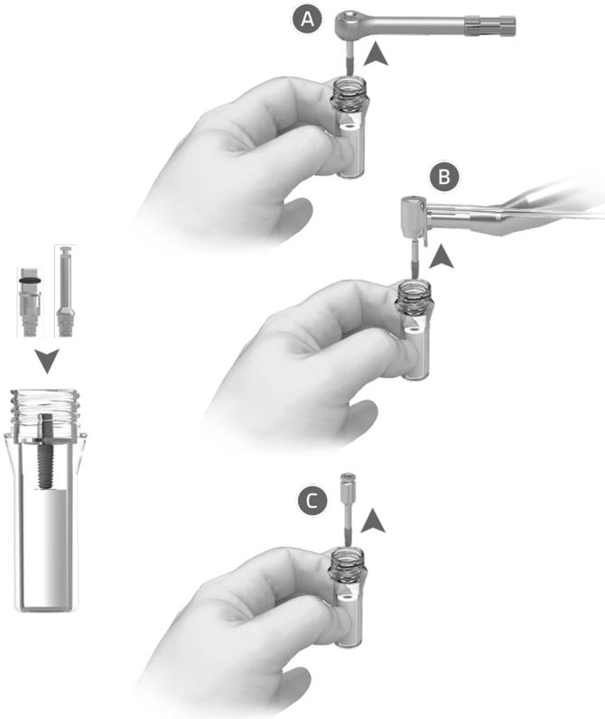
**EN** Manually hold the vial and insert the contra-angle or ratchet adapter into the implant holder. Ensure fixation of the adapter and remove the implant from the vial in the vertical direction.
